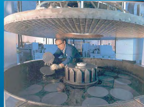
Wafers Lapping Process (Flatness Tolerance < 1micron for 1000 Cm 2 Surface Area of 300 mm Diameter Wafers).
